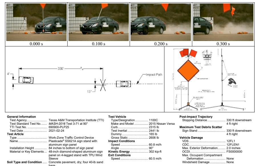
Figure 5.6. Summary of Results for *MASH-2016* Test 3-71 at 90 Degrees on Plasticade® SS621A Sign Stand with Aluminum Sign Panel Mounted at 84 inches.
