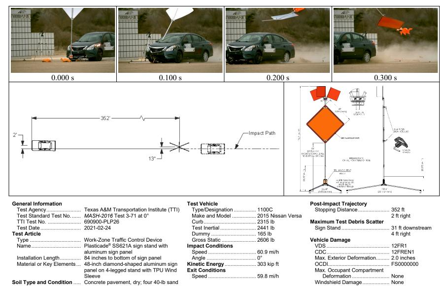
Figure 6.6. Summary of Results for *MASH* Test 3-71 at 0 Degrees on Plasticade® SS621A Sign Stand with Aluminum Sign Panel Mounted at 84 inches.
