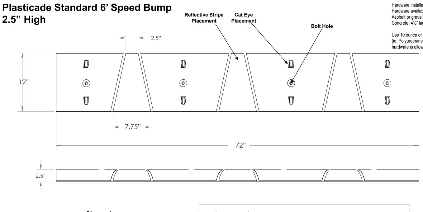
Hardware installation holes are drilled with a ½" drill bit. Hardware available:
