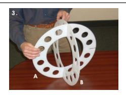
Stand the assembled section upright (intersections at bottom and top)
