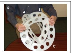
Position the assembled section and slightly bend the <u>all inside</u> ring to allow easy interlocking of the first pair of slots
