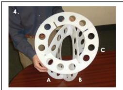
Place the <u>all inside</u> ring over the assembled section,
