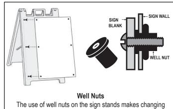
signs easier by providing permanent mounting holes
