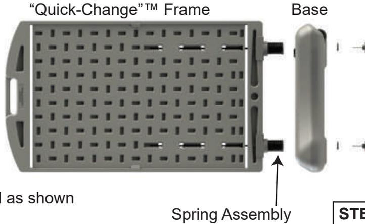
1. Lay frame on its side and base on end as shown
