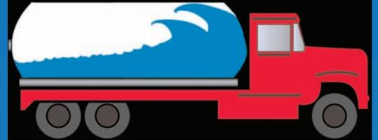
Wave forms inside tank when the truck starts or stops, creating a dangerous push that can destabilize the vehicle
