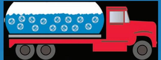
With Liquid Surge Stabilizers inside the tank, the upsurge of liquid is eliminated, improving the handling of the vehicle
